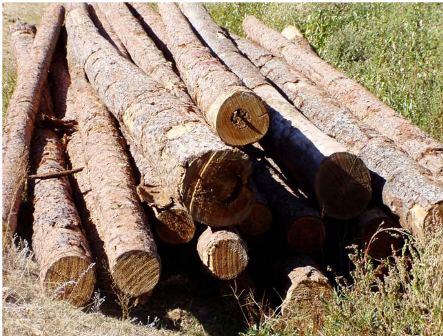
Photo A 2. Logs (15 m length x 0.5 m diameter) used in constructing triangular ramp-log structure on the Kettle River in 2008.
