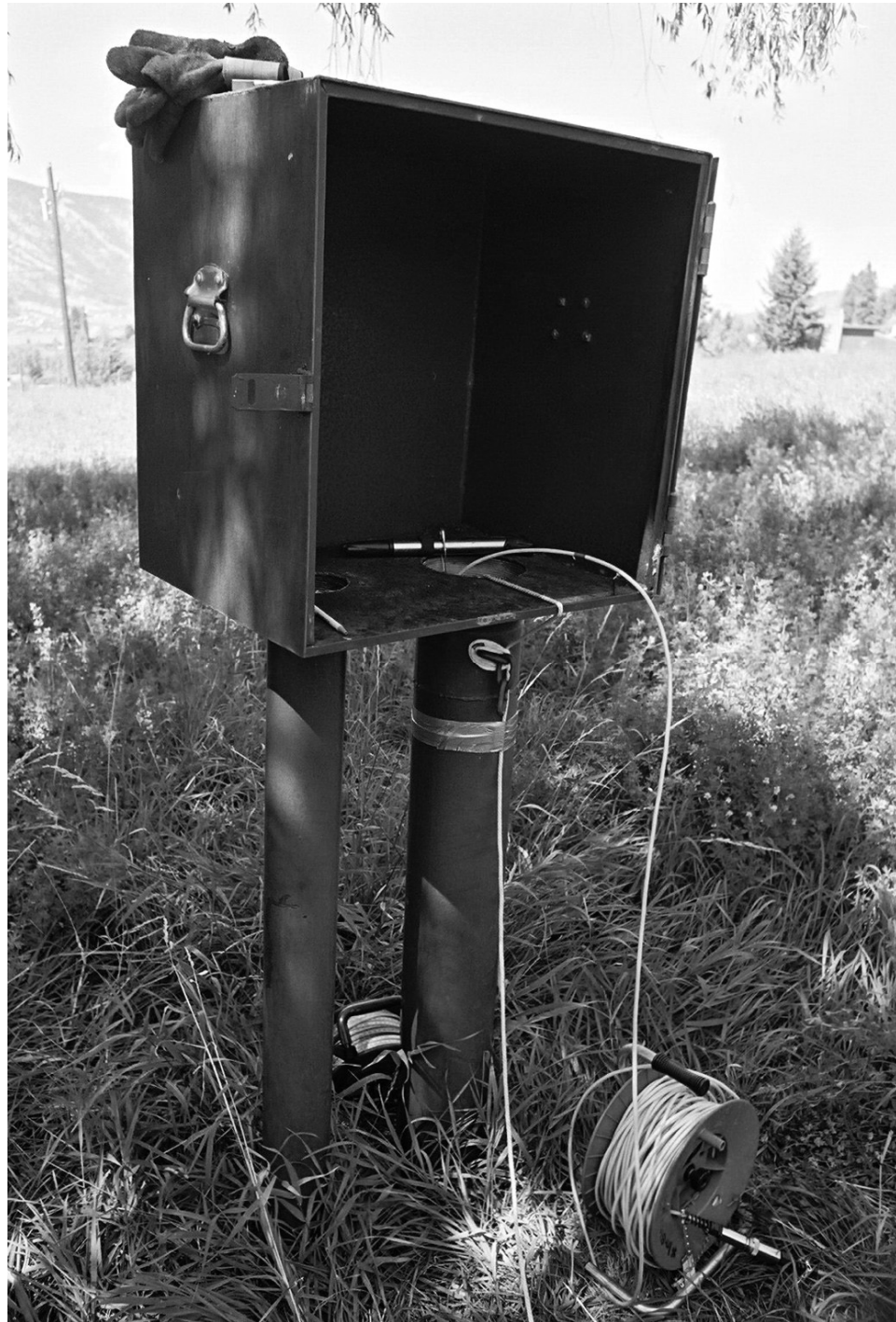
Figure 3.3 An observation well with a protective housing at the top of the casing. A slug test was in progress at the time the photograph was taken.
