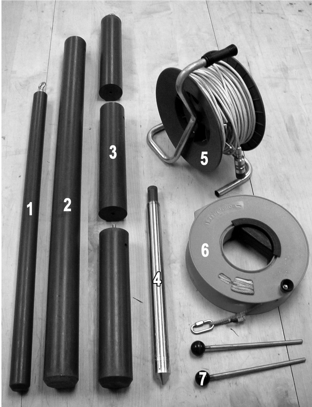
Figure 3.4 Slug testing apparatus used in the Okanagan Basin. (1) 1.25" diameter slug used in 2" wells; (2) 45" long section of 3" diameter slug assembly used in 6" or larger wells; (3) 15" long sections of 3" slug assembly; (4) TROLL 4000 data logger / pressure transducer; (5) 40m data cable; (6) nylon rope; (7) assembly pins.
