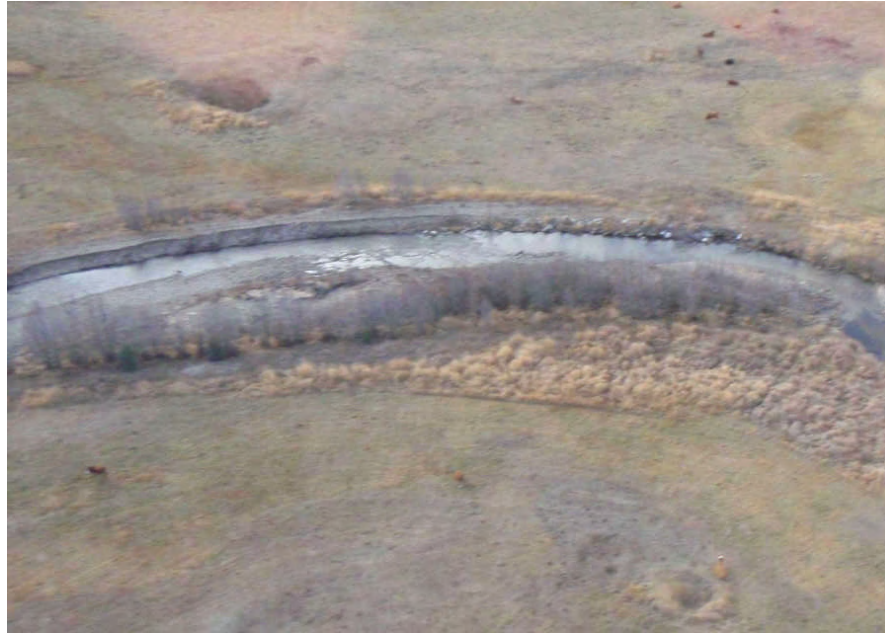
Photo 2. Cleared glaciofluvial/fluvial floodplain in Lower Trout Residual (Reach 9). Note long eroding unprotected bank.
