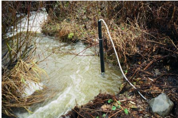
Figure 3. Example of size of stream monitored and instrument set-up for measurement of turbidity. Note water is turbid as a result of rainstorm.
