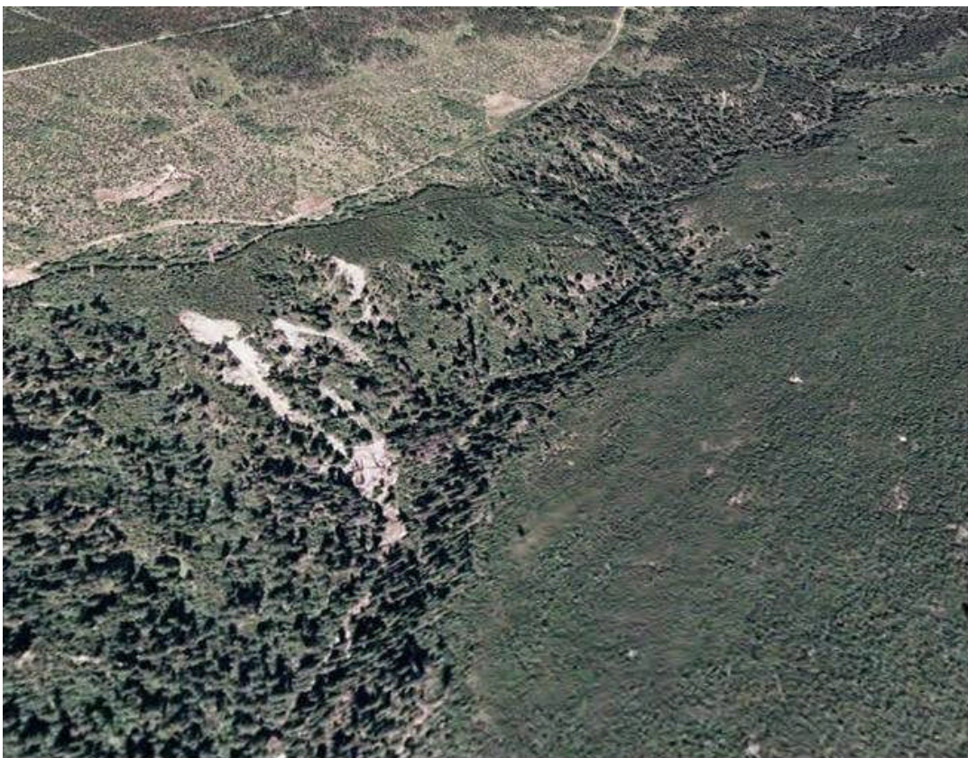
Photo 4. Google image of Landslide 1 from 2004 photography; still contributing some sediment to Penticton Creek mainstem. Smaller upstream slides are largely revegetated.
