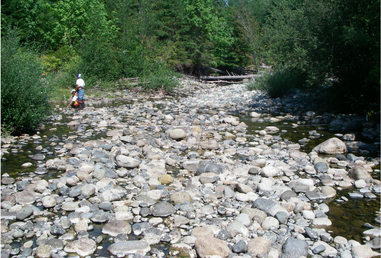
S. Englishman/Shelton : Measuring stream flows and rearing habitat conditions with Nanoose First Nation fisheries staff in the South Englishman River during the July 2009 drought. Total discharge was measured at 18 litres/second, or just 0.6% of mean annual discharge for this sub-basin (20%MAD is provincial ideal).
