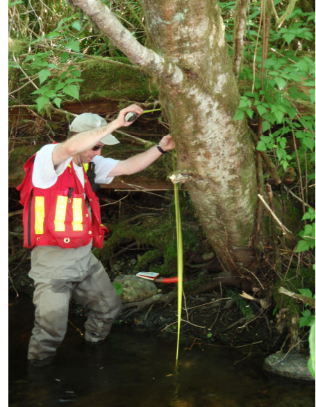
Keogh River : Data logger installed June 4, 2009 and used to record daily water levels on lower Keogh River; measuring the location for the gauging station housing.
