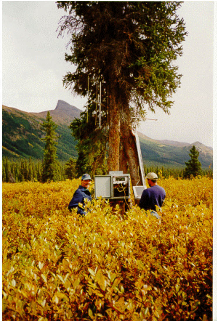
Figure 12. The fixed receiver station at the outlet of Mud Lake, immediately downstream of Sustut Lake. Note antennas mounted on trees, solar panel at right (in profile) and waterproof enclosure box housing receiver and 12 volt battery. The receiver is being downloaded to a laptop computer.
