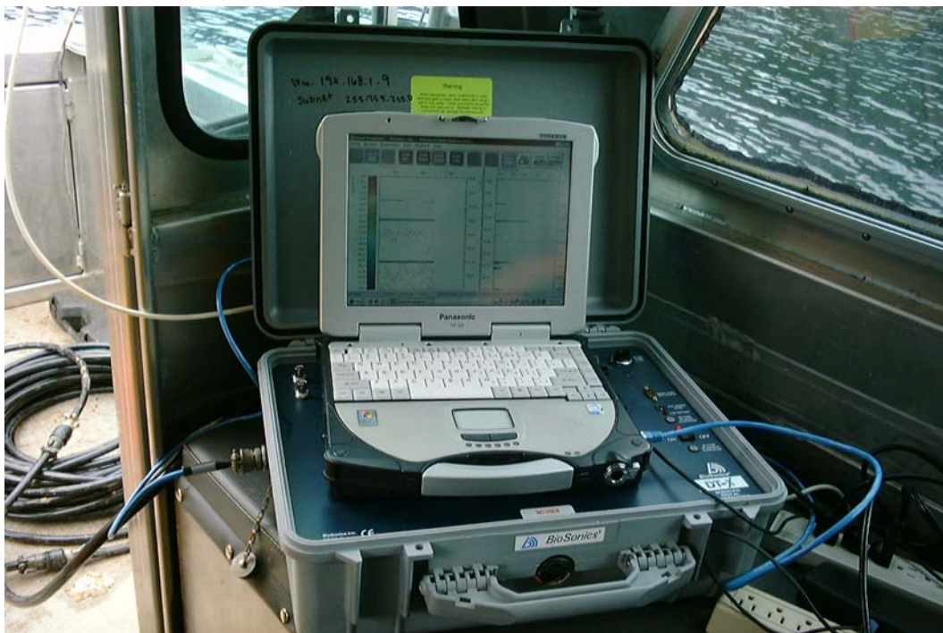
Photo 1. Echoprocessor used for hydroacoustic sampling on Coquitlam Reservoir, 2005.
