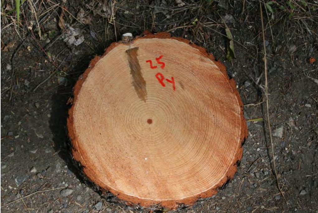
Figure 8. Sampled ponderosa pine (tree #25, Jones Cr. site) showing outline of inoculum dowel completely encased in pitch. Note there is no staining or any other indication of early decay in this region.
