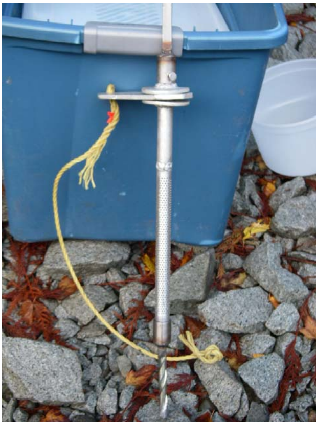
Photo 2. One of ten pipe incubators used to assess incubation survival of chinook eggs in the spawning platform in the Puntledge River Headpond 2006/07.
