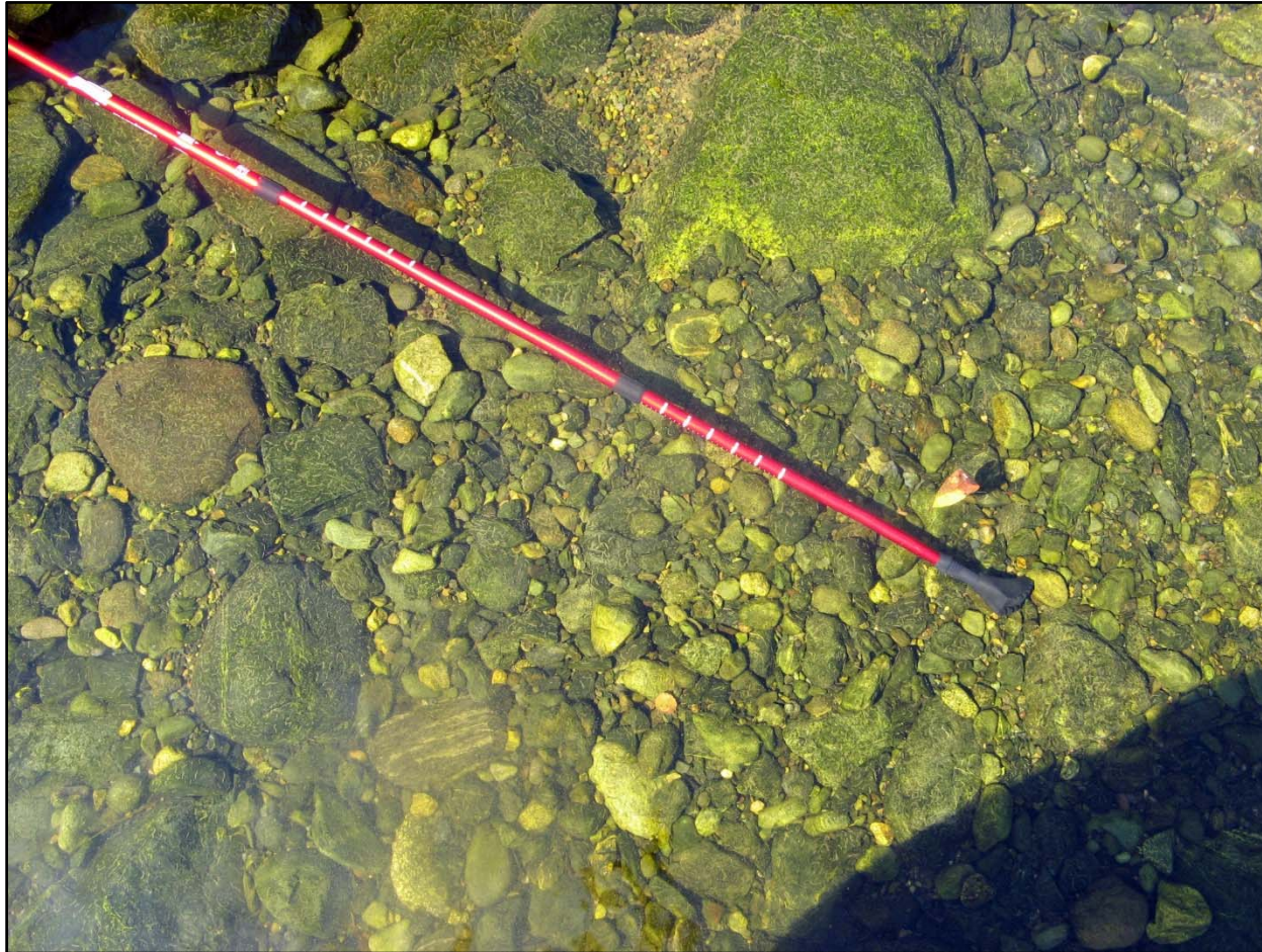
Photo 4. Close-up view of gravel composition of the continuous gravel pad (September 9, 2013). White bands on the walking stick are 2.5 cm.
