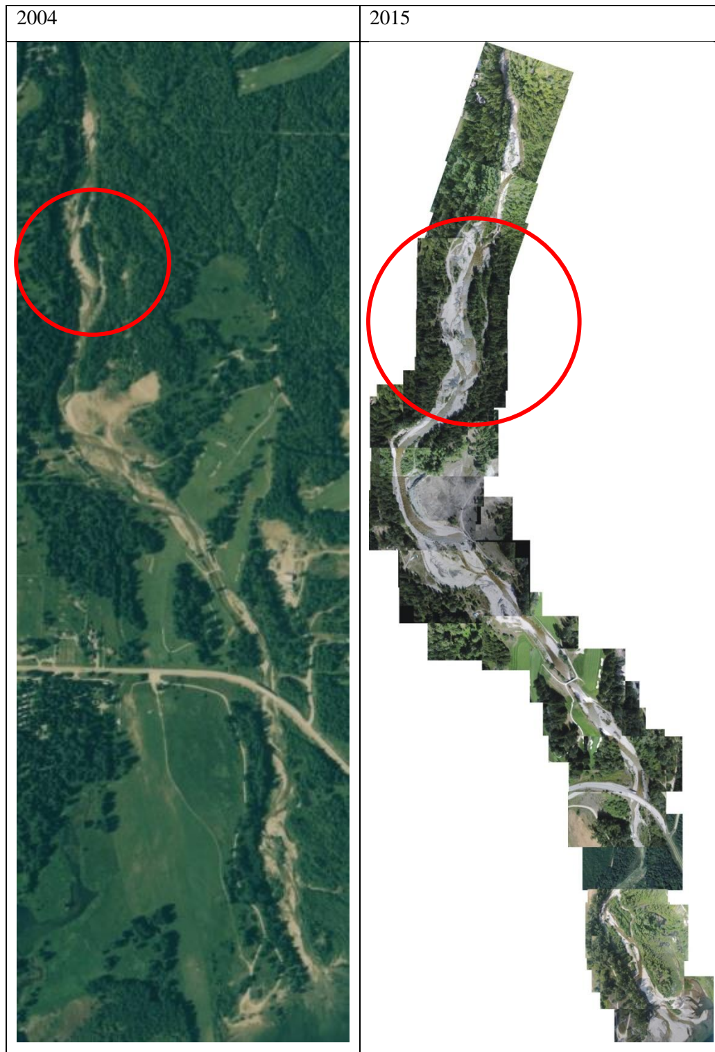
Figure 4. Larger scale comparison between 2004 air photograph and 2015 drone imagery shows that the disturbance associated with the 2012/2013 floods was greatest in the area upstream from the golf course gravel pit.
