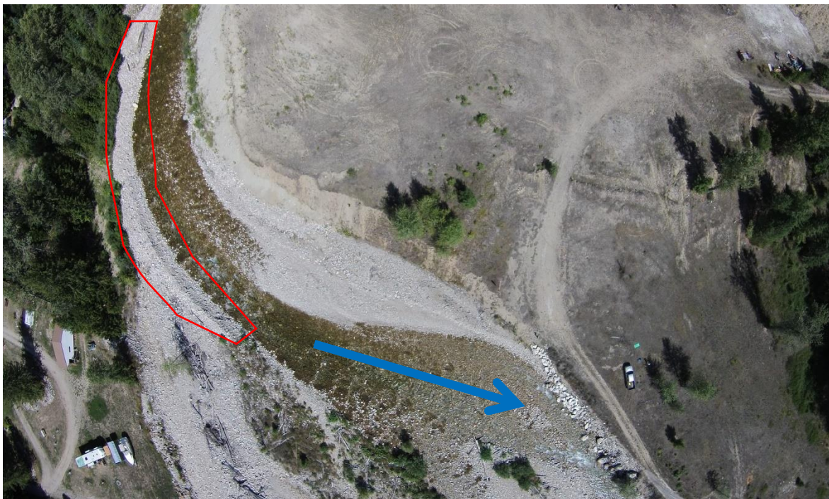
Photo 15. Looking down at approximately 100 meters of berm that is contributing sediment and creating scour along opposite bank. Blue arrow shows location of flow being directed by the berm and the area on the opposite bank that is being eroded.
