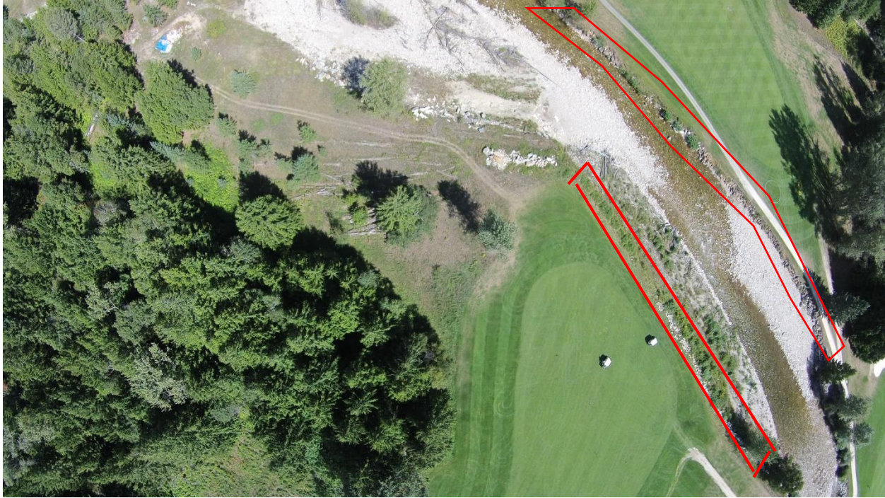
Photo 18. Erosion along fairway channel bank - east side
