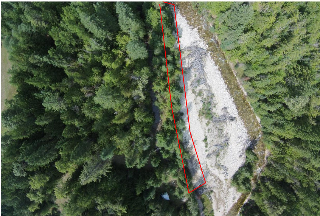
Photo 13. Looking down at approximately 100 meters of raveling bank on channel side of spawning channel.
