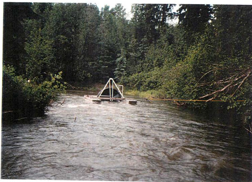
Figure 2. Example of common rotary screw trap setting at Toboggan Creek in the spring of 1998. Note trap position which provided good trap performance by intercepting high velocity water.
