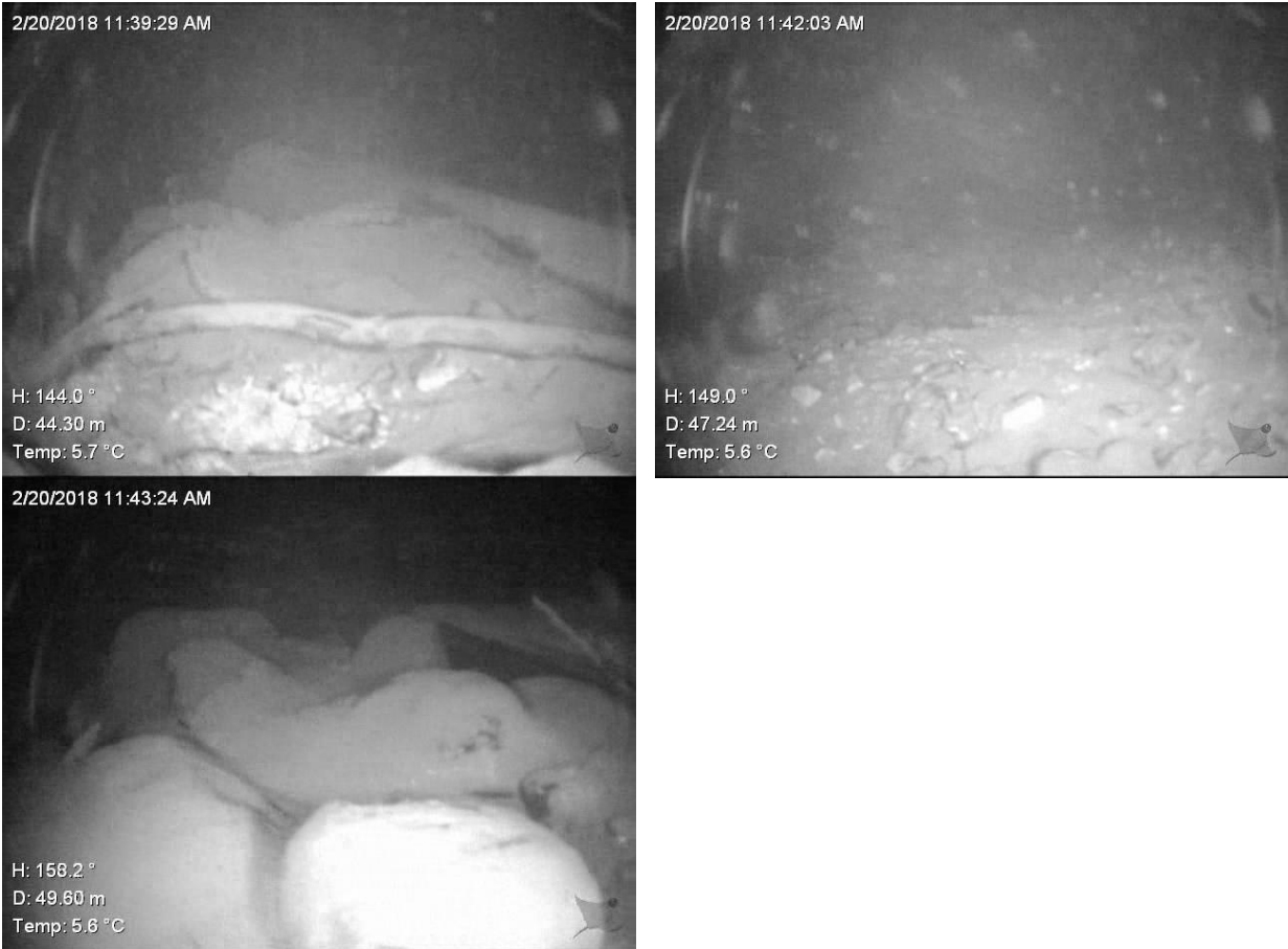
Figure 4-16 Remote operated vehicle (ROV) imagery showing a cleaned redd (top left) as well as example substrate types (top right: cobble gravel with embeddedness 41-80%, bottom left: cobble with embeddedness 41-80%) in Area G of Alouette Reservoir, BC.
