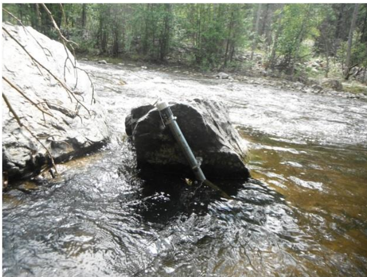
Figure 6: Hydrometric station showing a stilling well anchored to a boulder in a relatively calm pool. An unvented pressure transducer is suspended inside the stilling well. Photo credit: ONA.
