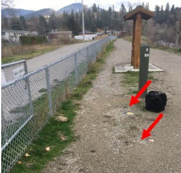
Figure 7: Piezometers flush-mounted with the ground surface near the Hollywood Road hydrometric station. Unvented pressure transducers are suspended in the piezometers. Photo credit: Piteau Associates.
