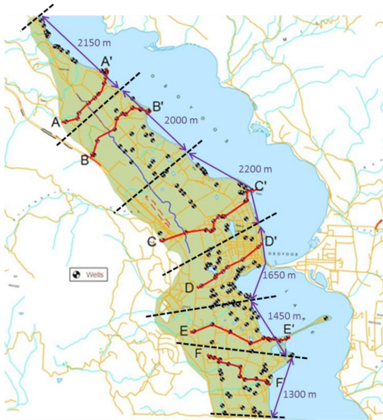
Figure 13: Aquifer sections used in Darcy flux calculations.
