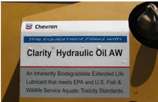
Photo 3. Fish safe hydraulic fluid used by instream machinery.
