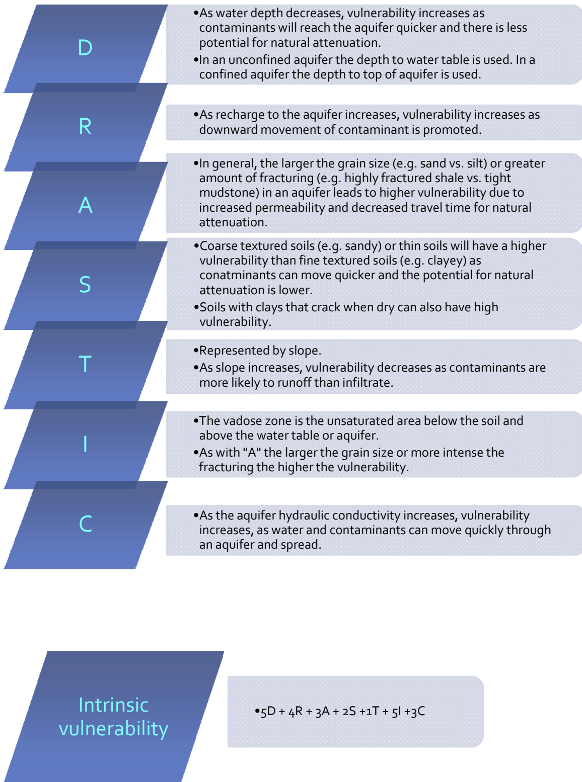
Figure 3: DRASTIC parameter descriptions and combination to form the final intrinsic vulnerability map
