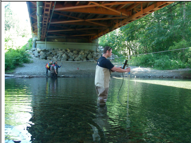
3. BCCF & WSC staff measuring discharge at WSC stn# o8HBo02 (Englishman R near Parksville; July 2010)
