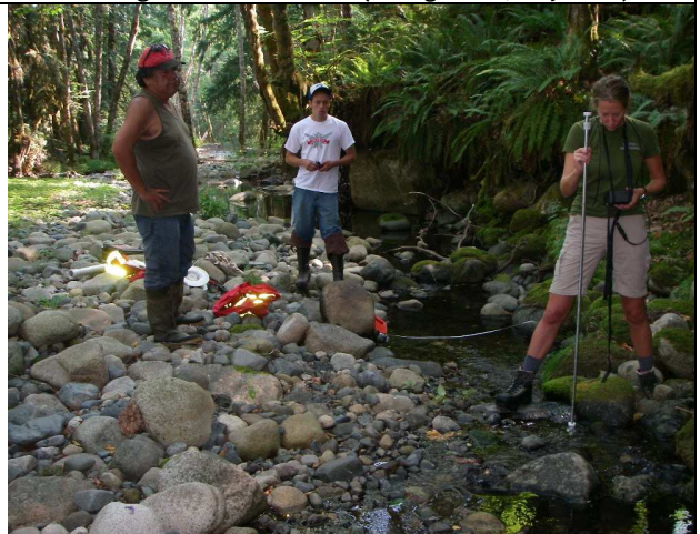
6. Nanoose First Nation and BCCF staff measuring flow in Centre Cr, the South Englishman's only anadromous trib.
