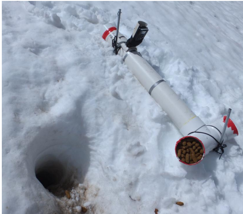
A feeder installed at the Sunrise Lake colony in the spring, 2013. The remote camera sits in a bracket at the top of the feeder (C. White).
