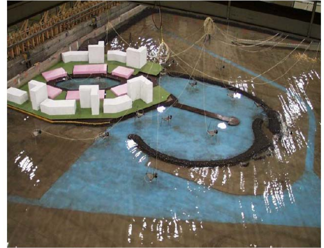
Figure 5.47: Physical model investigation of hydrodynamics in a new marina (National Research Council Canada)
