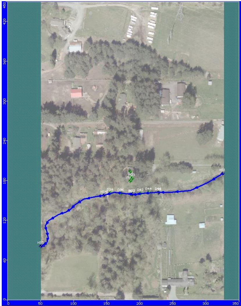
Figure 36: Numerical model domain in plan view showing the location of the stream boundary condition (blue), and the wells, instream piezometers and hydrometric stations used for calibration. The horizontal grid is not shown for clarity purposes.
