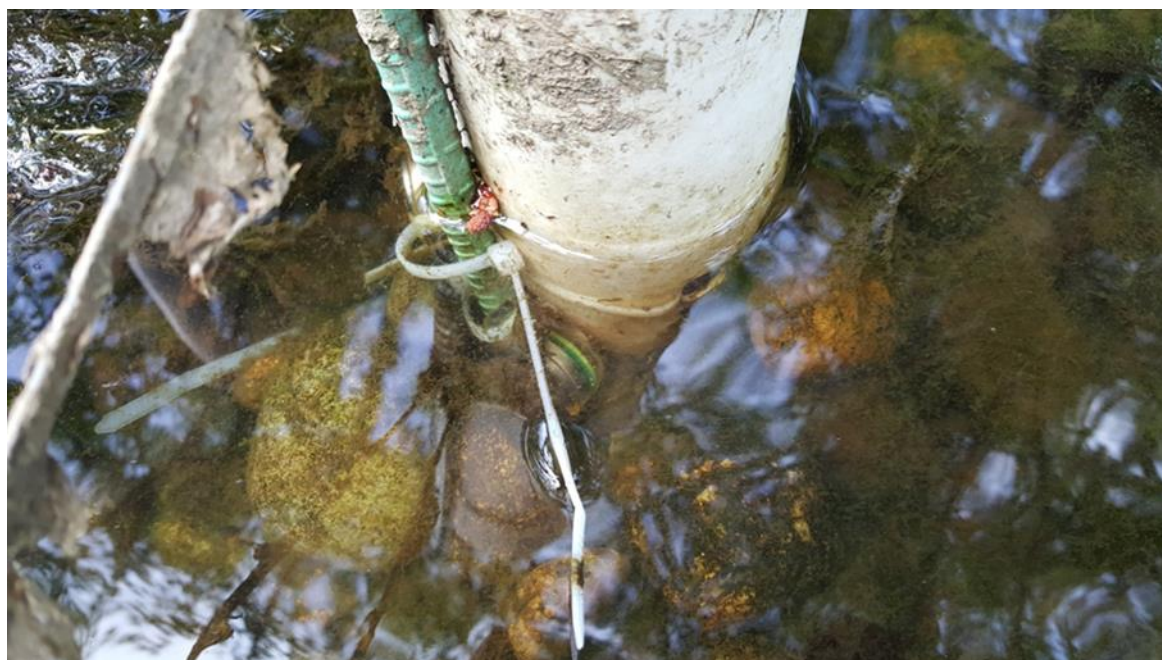
Figure 13: TidBit temperature logger installed attached to the rebar on the outside of the PVC tubing for the pumping test. Background TidBits are installed inside the tube.
