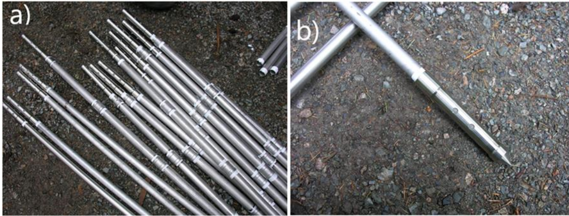
Figure 10: a) Assembled links of the piezometers before installation; b) the screened interval of the piezometers.
