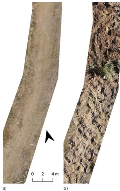
Figure 8.11. A comparison of part of the road surface of flight 04 a) before and b) after treatment. The road surface decompacted, coarse woody debris stacked across the road, and the access management ditch has been enlarged.
