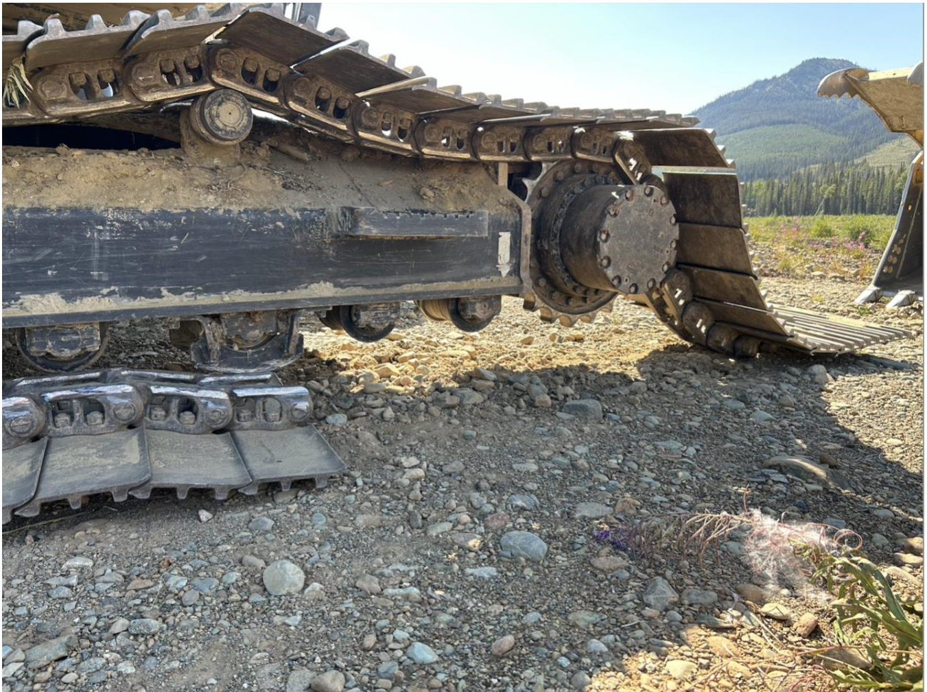
Figure 4.1: Photo of the broken track link on the John Deere 210G excavator that was being used for restoration in 2024.
