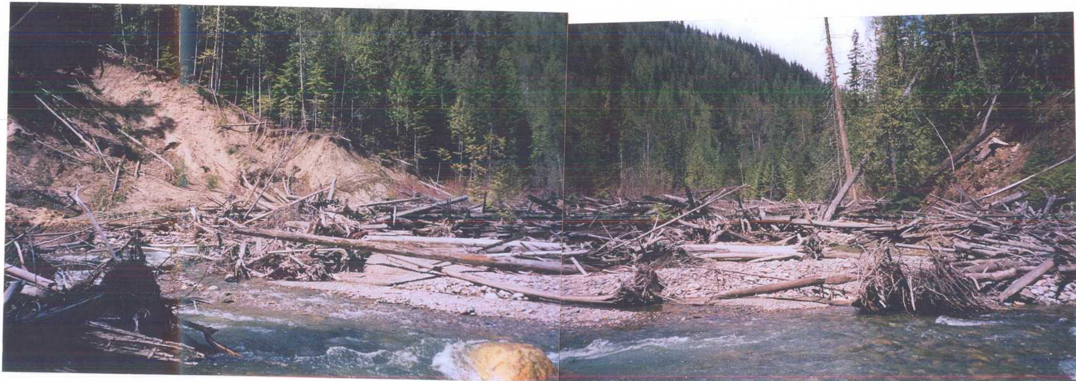
Photo 5. Lowermost debris jam on reach R4. The channel has eroded around the jam on the left side of the photo re-activating a large slope failure in glacio-fluvial and lacustrine terrace deposits. This jam is approximately 75 m width and 3 m high.
