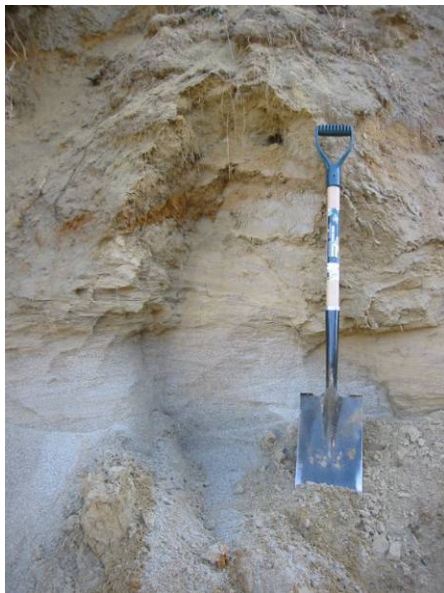
Photo 8. Bedding planes of silt and sand in a massive glaciofluvial deposit in the Albreda project area.
