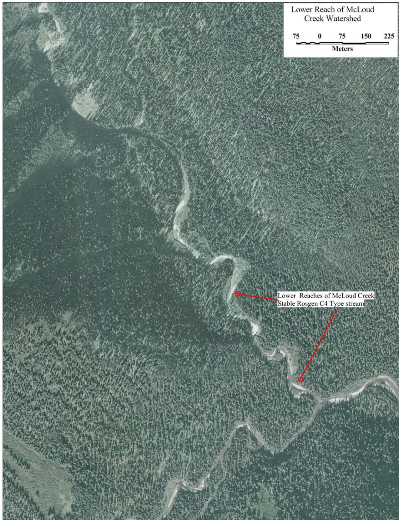
Figure 24. Lower reaches of Macleod Creek. At this location, this is a stable C4 type stream
