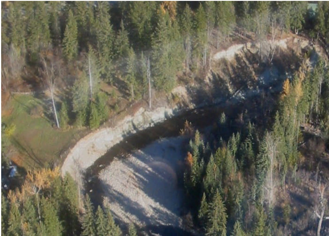
Photo 8. Mission Creek (Reach 4) bank erosion of thick sand, gravel and cobble glaciofluvial and fluvial sediments.
