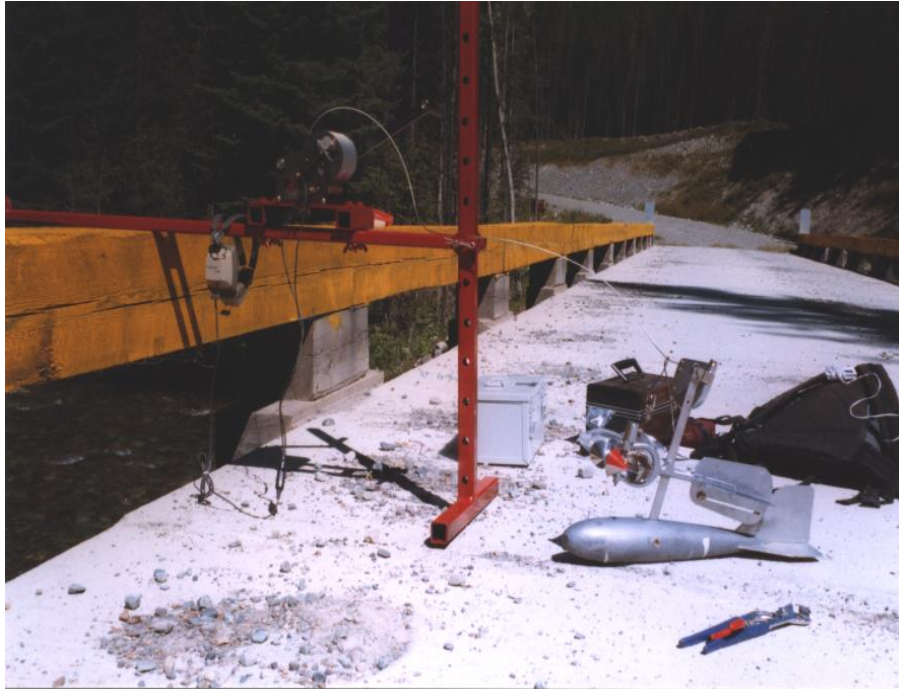
Figure 3.2.1 Bridge crane and sounding reel suspension used to raise and lower the Price AA velocity meter needed to calculate discharge for the Wigwam River.
