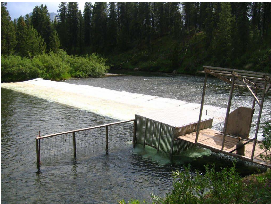
Figure 3. Photograph steelhead enumeration fence assembly (a) and fence in operation. (b), 2008. Courtesy of Brome and Leaf Steffey.
