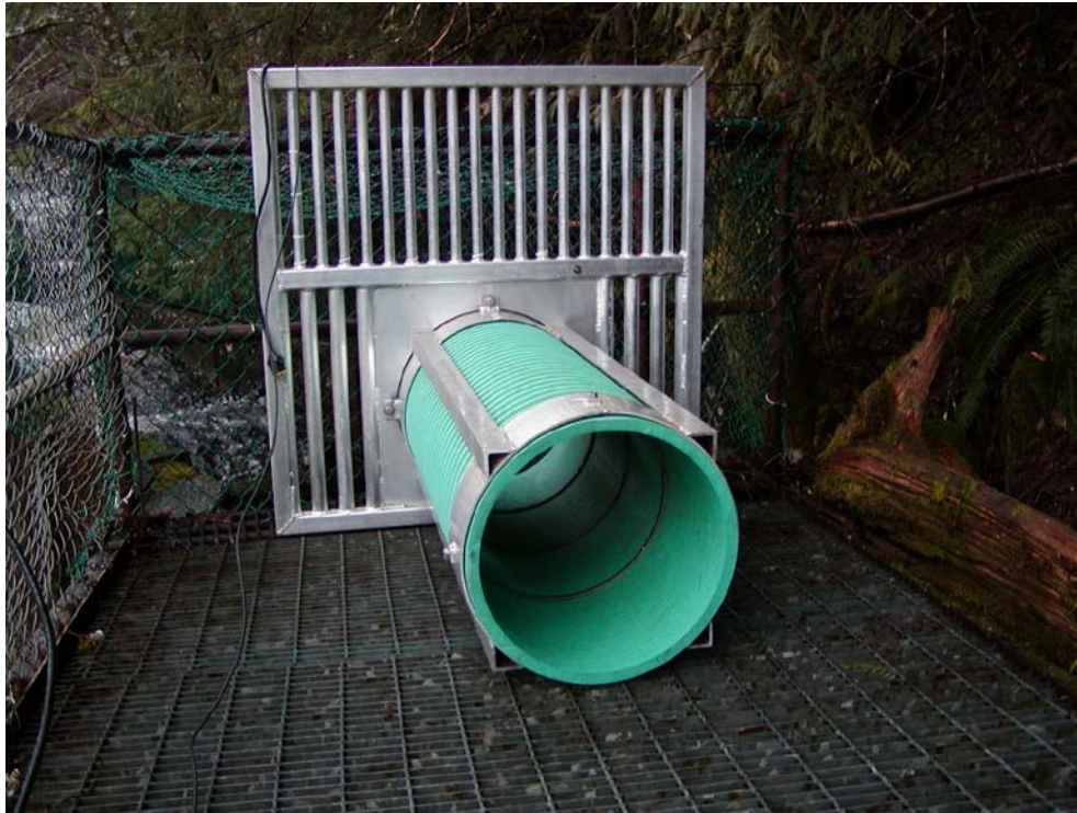
Picture 1. Kloiya River resistivity counter tube
