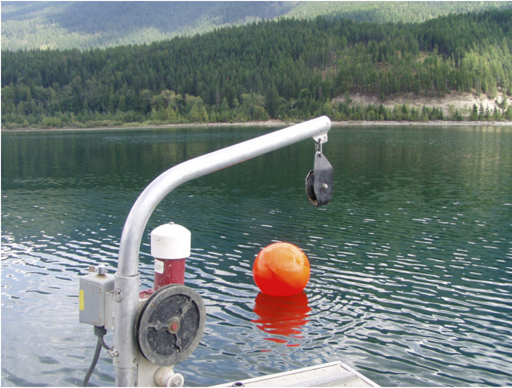
Photo 1. Deploying a Vemco VR2W receiver near the mouth of the Lardeau/Duncan Rivers in August 2007.
