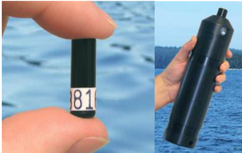
Photo 2. V7 acoustic tag (left) transmitter and a VR2W receiver (right) used on the Lardeau River in 2007
