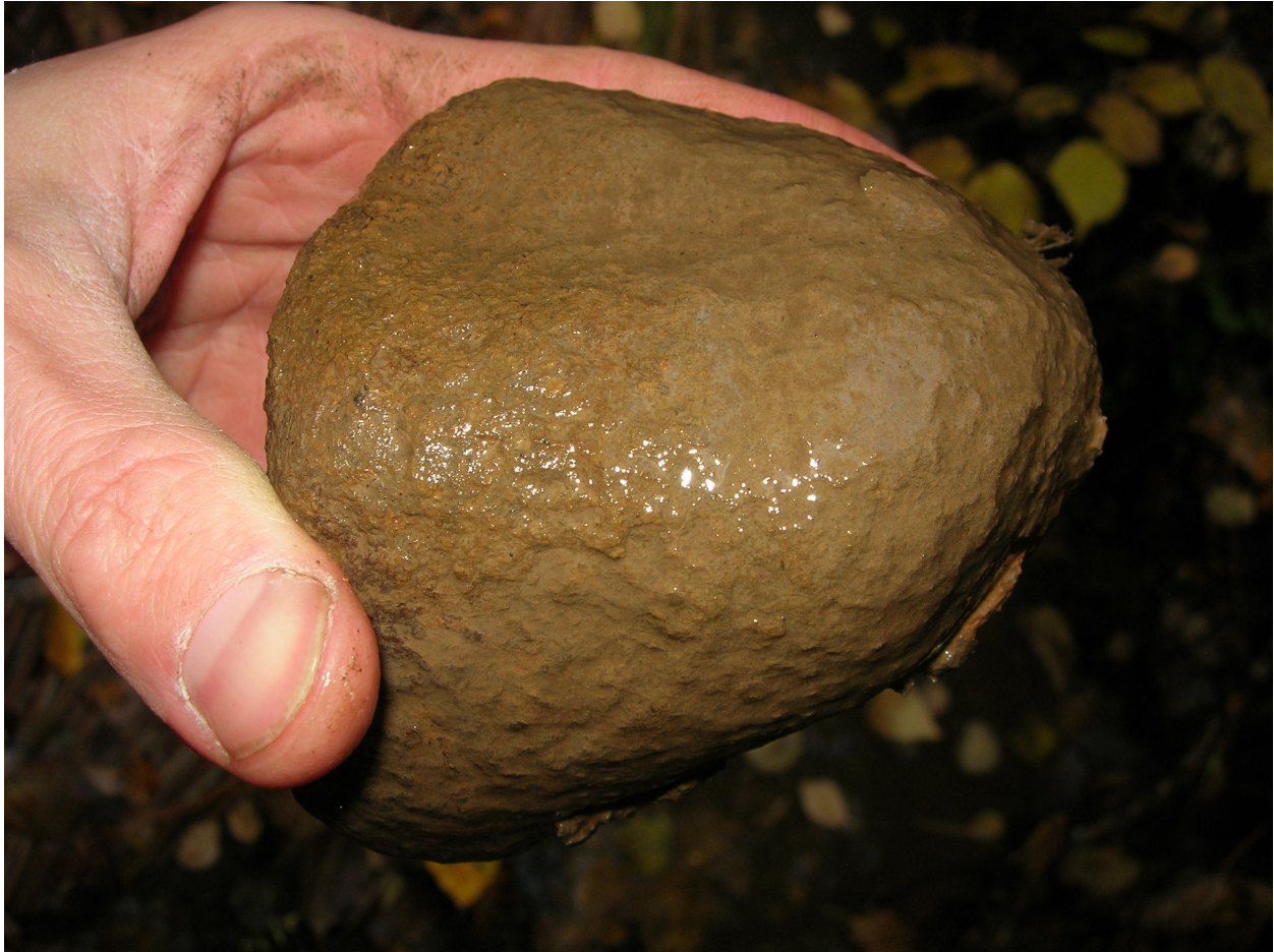
Photo 12: Site 270 - Looking at silt covered cobble downstream of culvert as evidence of high levels of past sedimentation.
