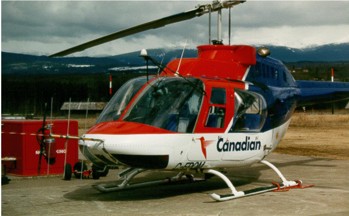
**Figure 5. Helicopter used for tracking flights showing the location of telemetry antenna, mounted on the aircraft's high frequency antenna, and GPS antenna (white dome over front window).**
