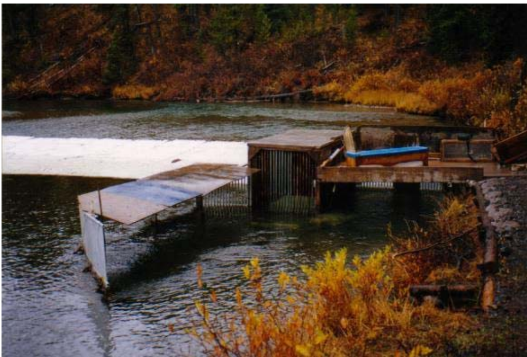
Figure 3. Aerial photograph of the steelhead enumeration fence looking downstream (a) and photograph of the fence from the trail on the right bank (b) of the Sustut River, 1998.
