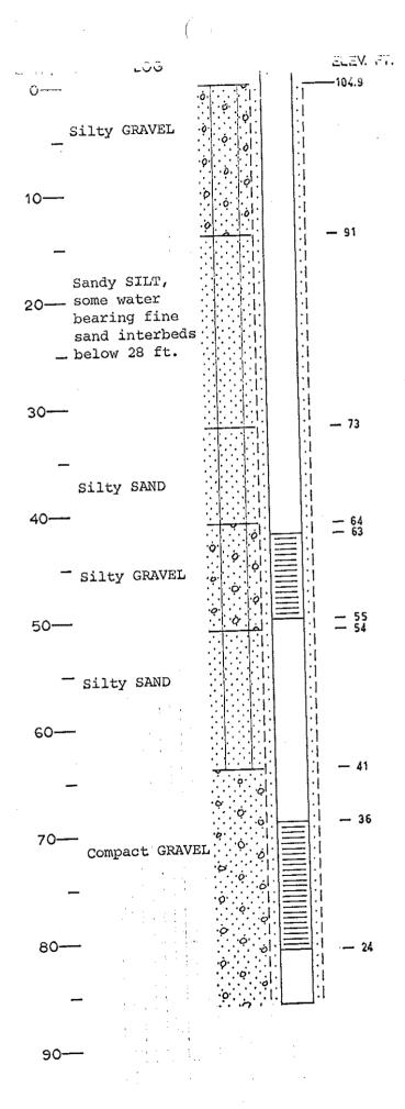
Hole 8-inch diameter drilled and cased to 86 ft. depth.
