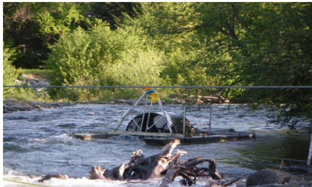
Figure 4. Rotary screw trap (RST) in operation on Gates Creek. Cable way visible across middle of figure.
