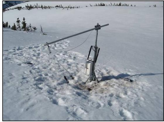
A weather station in the upper Ospika River drainage damaged by a grizzly bear in early spring.
