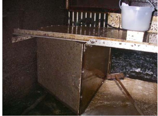
Photo 3. Camera tunnel installation in the Comox Dam fishway before cleaning, February 20, 2008. Plexiglass wall of tunnel is completely covered in sludge and macroinvertebrate growth.
