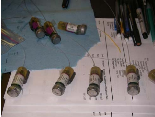
Photo 1. Conventional Lotek MCTF radio telemetry transmitters with temperature loggers attached on the end.
