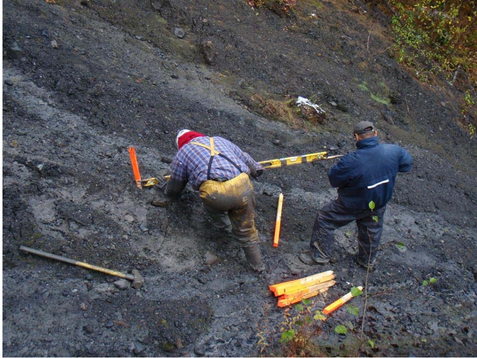
Photo 48: Line 1 stake placement using 2-meter level at Site 48 (October 17, 2008).
