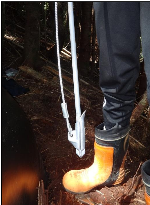
Figure 4. Anchor on pounding rod before installation.
