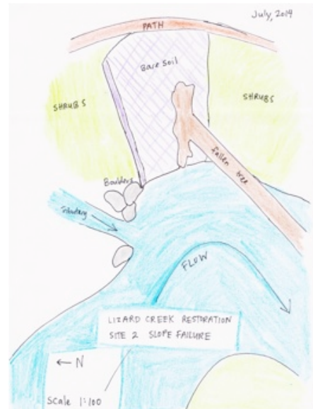
Figure 5- Site 2 Slope Failure Drawing
