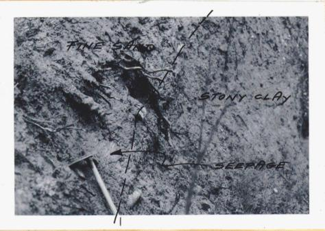
FINE SAND OVERLYING HARD STONY CLAY. NOTE SEEPAGE FROM SAND AT CONTACT.
