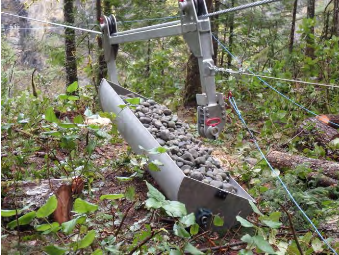
Photo 21. Failed trolley bucket, third load, March 24, 2016.
