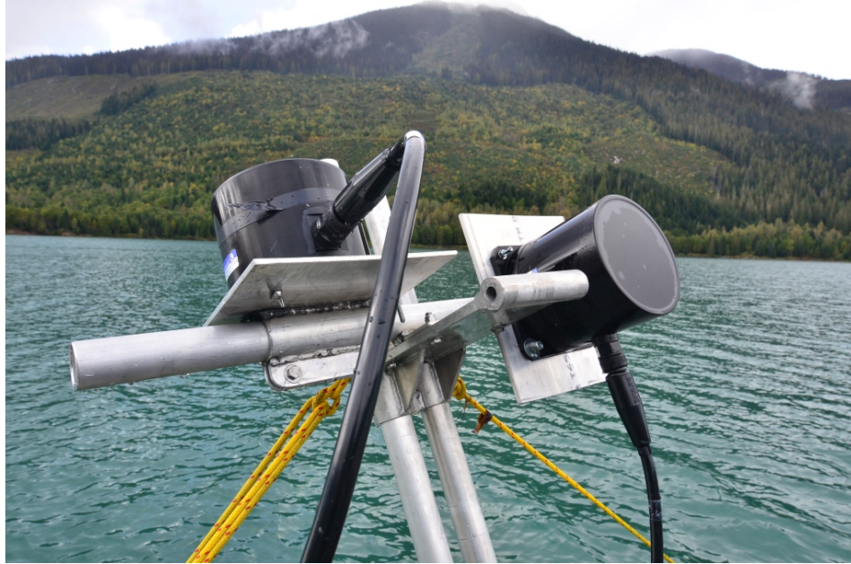
Figure 3 Set-up for the down-looking and the side-looking circular transducers used for the 2015 hydroacoustic surveys.
