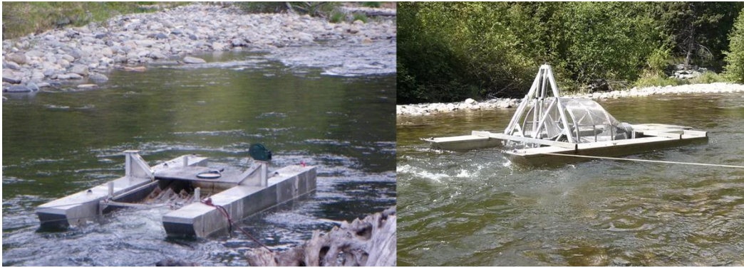
Figure 4. Inclined plane trap (left) and rotary screw trap (right) in Gates Creek.
