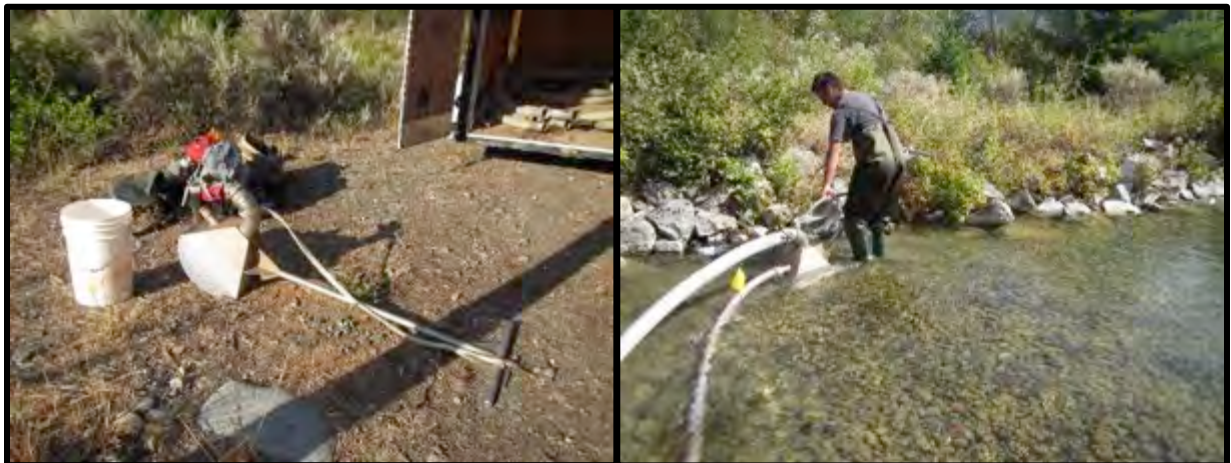
Figure 6 SandWand head (left) and equipment in operation Aug 2015
