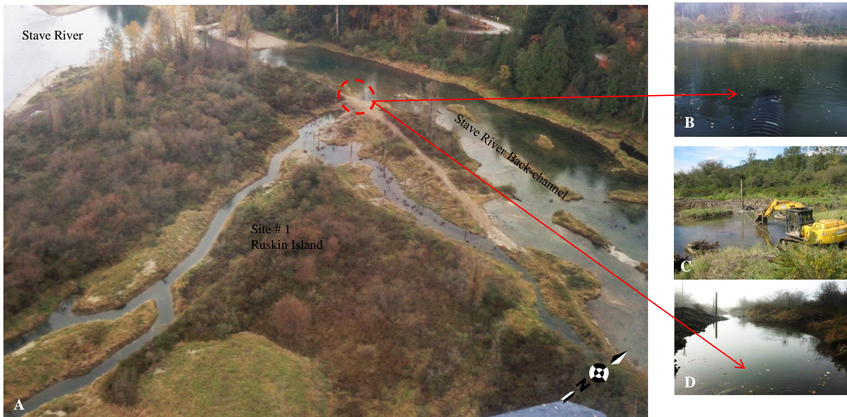
A. Air-photo of Ruskin Island showing location of intake replacement. B. New Boss 2000 intake installed north-view in the back-channel. C. Machine installing new intake and avoiding archaeological feature. D. New Boss 2000 intake installed south-view to newly constructed off-channel salmon habitat. C.
