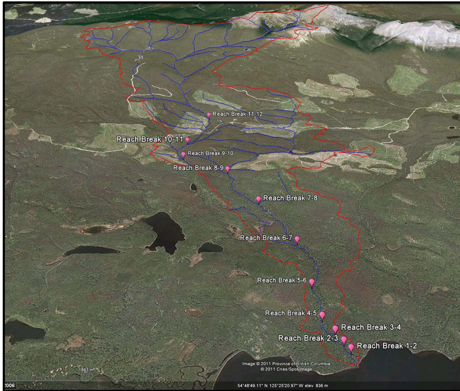
Figure 4. Identification of reach breaks along the mainstem of the lower Paula Creek watershed
