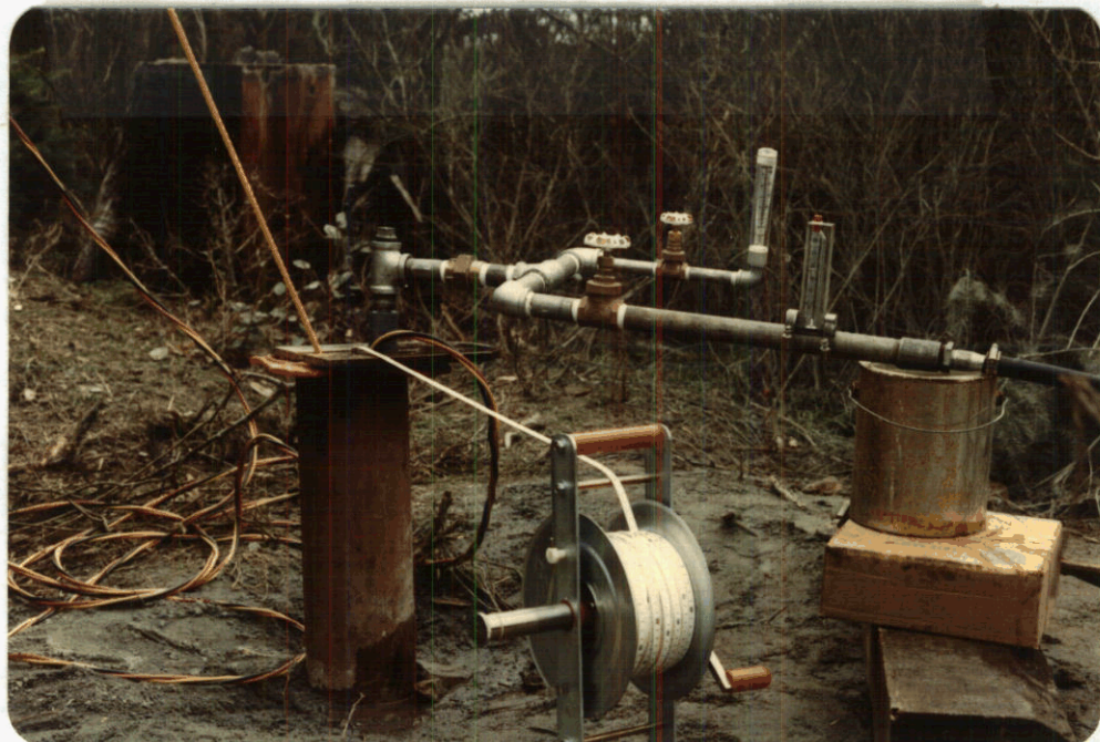
6. Observation Well WR 258-60 Galiano Island (south) Pumping test flow meter and water level indicator
